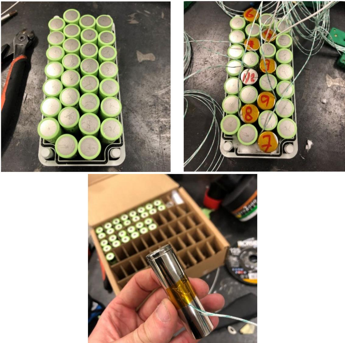
Figure 6 The contents of the battery pack and placement of thermocouples.
