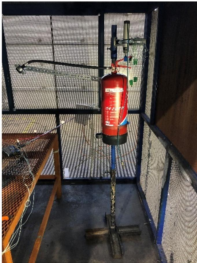
Figure 3 Fixture for the fire extinguisher including pneumatic cylinder for remote activation
