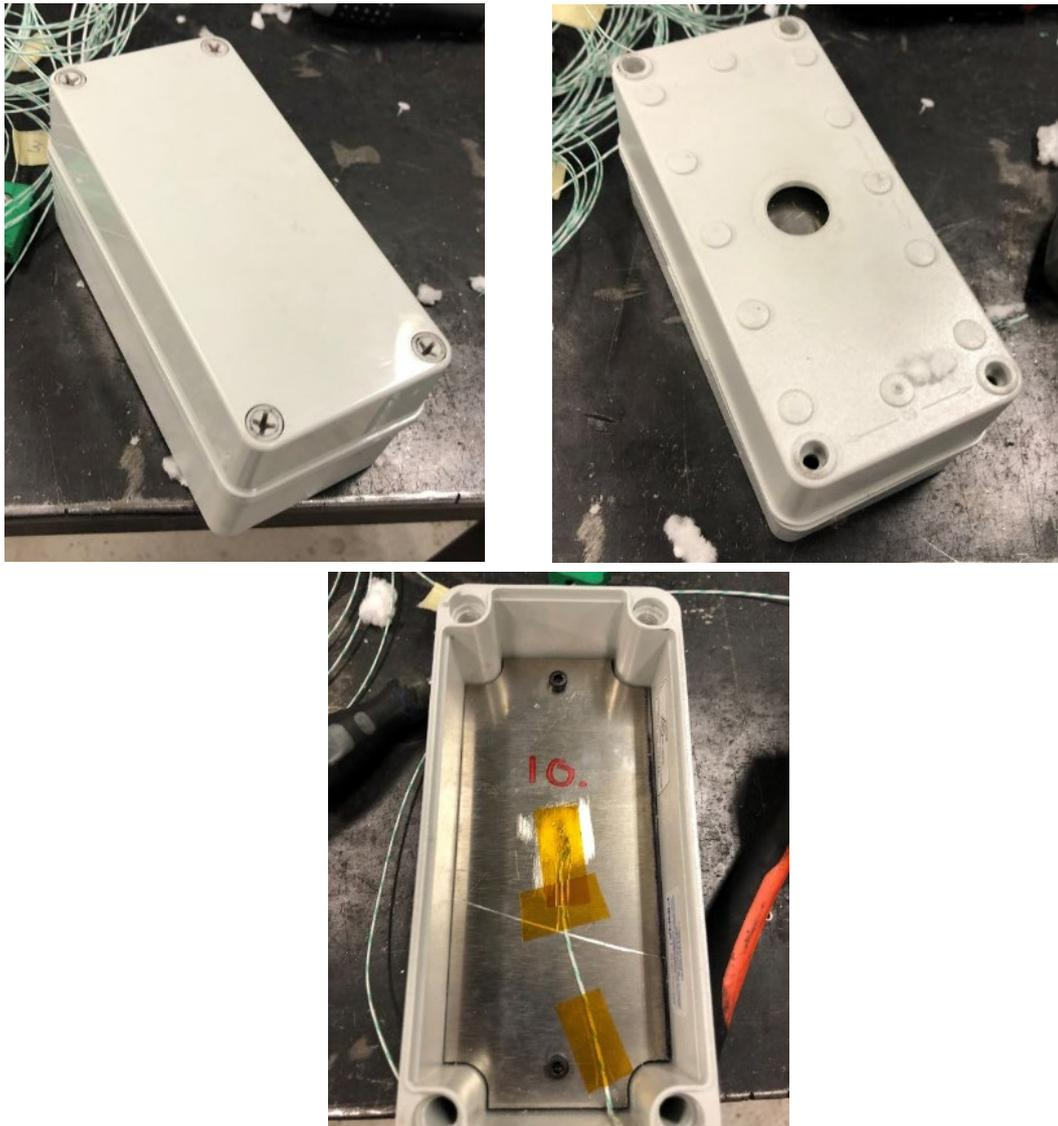
Figure 5 Overview of the pack, the opening, and the steel plate mounted within.
